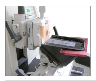
The vessel is filled with water up to the blade. After trimming, remove the section waste from the tray and create the sections to be prepared. The sections floating on the surface of the water can be removed using the glass slide.
